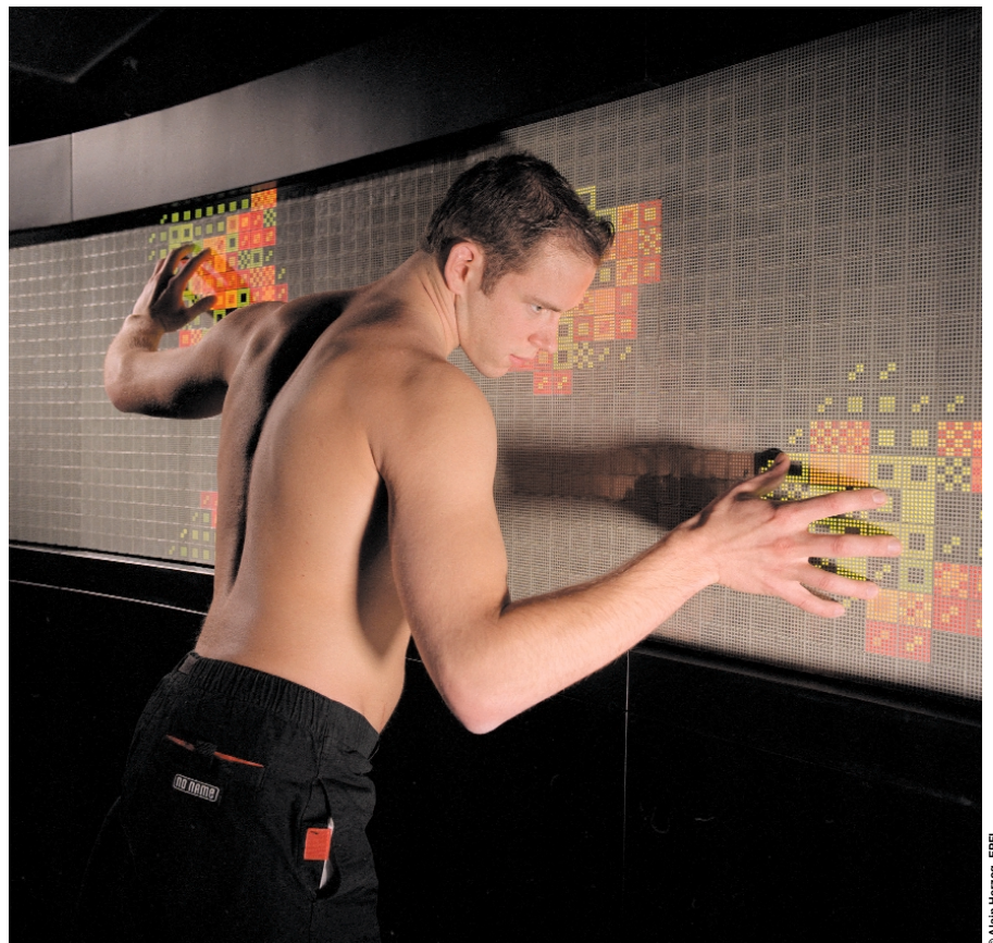
The BioWall: A self-repairing cellular computing machine built at the Swiss Federal Institute of Technology in Lausanne (EPFL).
