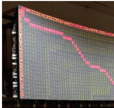
Figure 13 – The Needleman-Wunsch algorithm implemented on the BioWall
